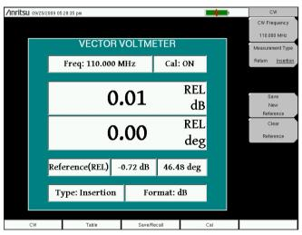
Figure 12. Comparing cable parameters on phase and insertion loss is easy, as shown on this VVM display, with the relative differences in the middle and the original parameter values (gold standard unit) in the lower portion of the screen. The two cables are more phase matched as the relative difference between them becomes smaller.
