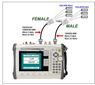
Figure 8. VNA Master's calibration procedures provide the zero-phase reference for later insertion-phase measurements. The calibration algorithm requires a through connection so it is important to set up a male-female interconnect scheme to ensure a precise zero-phase reference.
