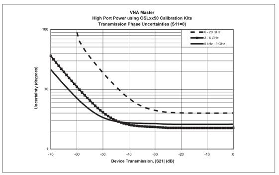
Figure 15. Phase measurement uncertainty for three different frequency ranges for the VNA Master are pictured in this graphic. Note that as the  $S_{21}$  insertion loss increases to 70 dB, the uncertainty increases, caused by trying to get phase information out of a much lower test signal.
